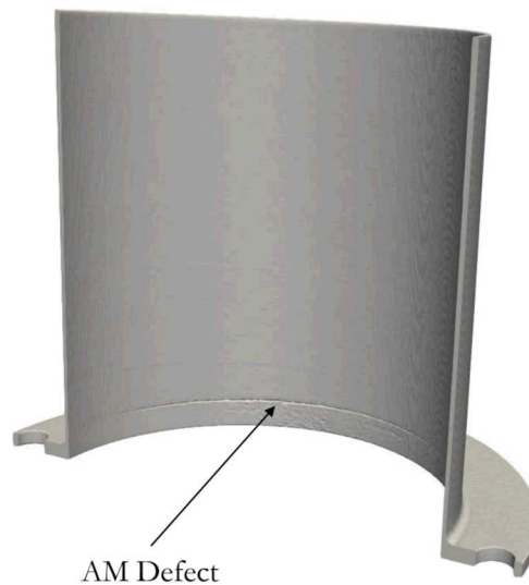
Fig. 1- Component with Defect on Inner Wall
