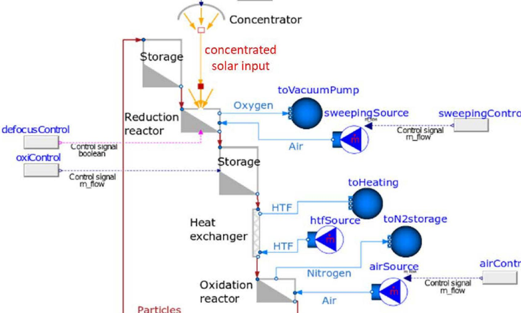
To calculate the annual amount of  $\text{N}_2$  produced from STAP under solar conditions, a system model of the  $\text{N}_2$  separation process has been developed. The model was implemented using Modelica. ([www.modelica.org/documents](http://www.modelica.org/documents))
