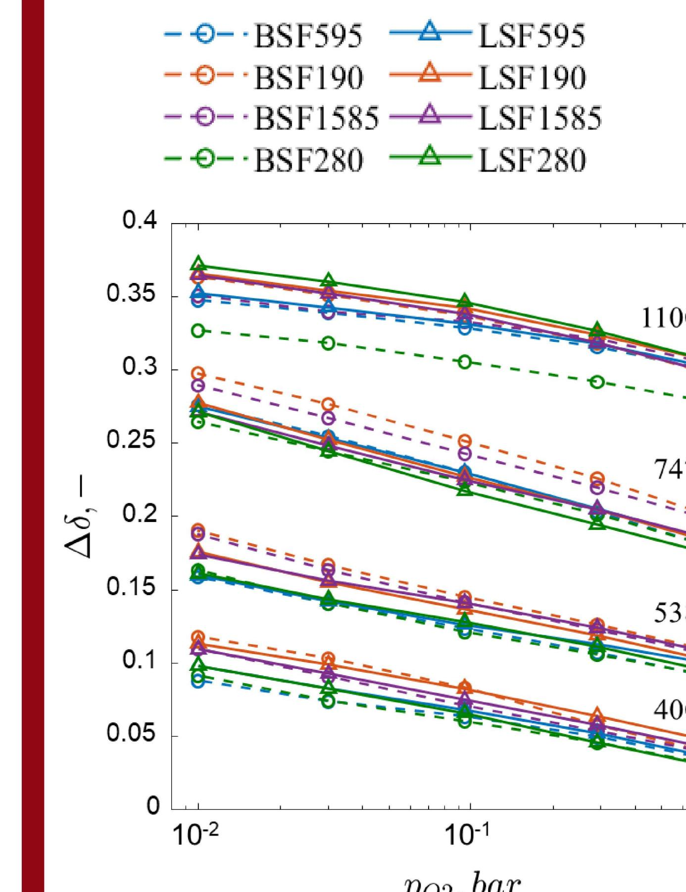
$\text{Ba}_x\text{Sr}_{1-x}\text{FeO}_{3-\delta}$  and  $\text{La}_x\text{Sr}_{1-x}\text{FeO}_{3-\delta}$  nonstoichiometry ( $x = 0.05, 0.1, 0.15, 0.2$ ) as a function of  $\text{O}_2$  partial pressure and temperature.
