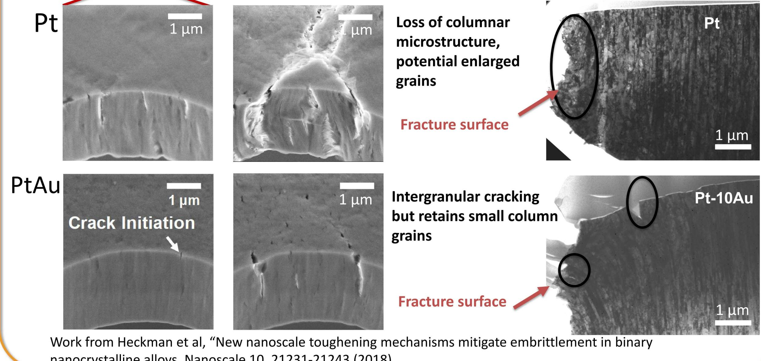
Work from Heckman et al., "New nanoscale toughening mechanisms mitigate embrittlement in binary nanocrystalline alloys," *Nanoscale* 10, 21231-21243 (2018).
