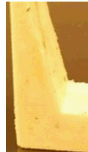
**Mechanism:** Spatial variations in density and extent of cure from manufacturing couple with cure shrinkage, thermal expansion, and confining conditions during cure to produce a complex residual stress state that relaxes over time.
