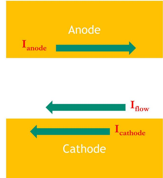
$$I_{\text{anode}} = I_{\text{cathode}} + I_{\text{flow}}$$
