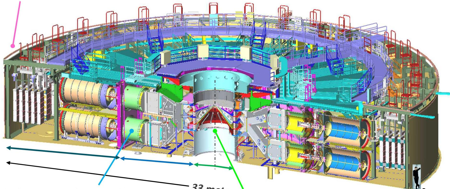
*pulse-forming section (400,000 gallons  $H_2O$ ): laser-triggered  $SF_6$  gas switches &  $H_2O$  spark-gap switches compress pulse to 100-1500 ns rise time, tri-plates reduce 36 lines to 18, convolute reduces further to 4 radial feed gaps*
