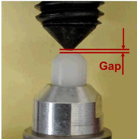
0.07mm Nonlinear Gap Connection
