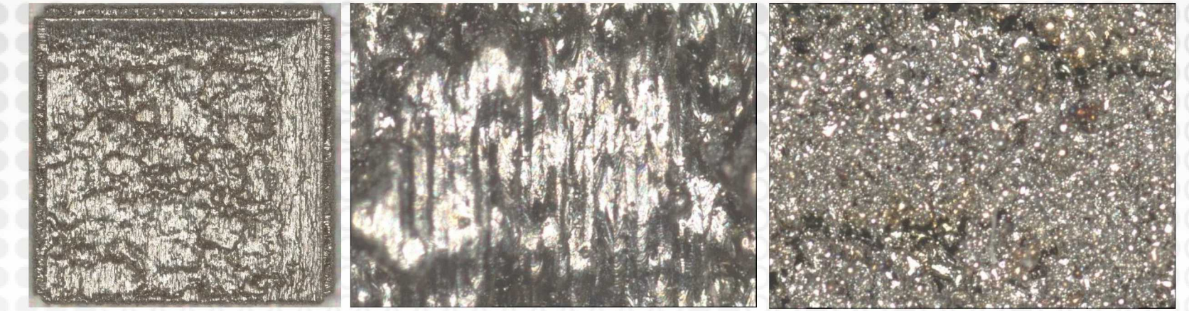
60.1W, 300mm/sec, top 891 \mu m PV form (left), top 73.8 \mu m S_a roughness (center), side 38.1 \mu m S_a roughness (right)
