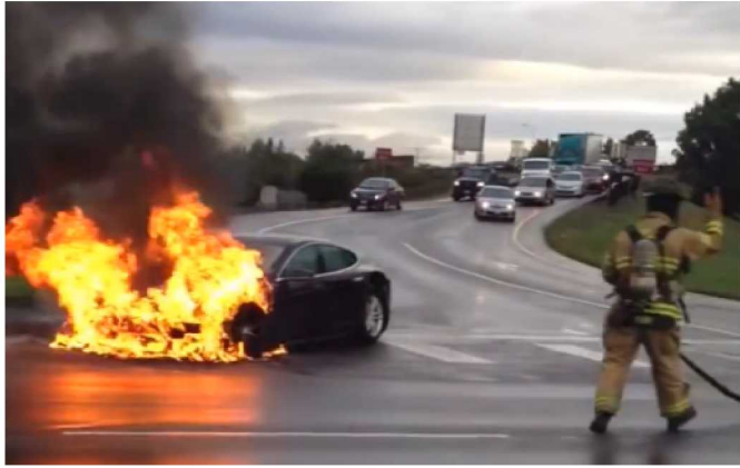
Tesla Model S fire in October 2013, where the fire was isolated to the front portion of the vehicle and did not propagate through the entire battery
