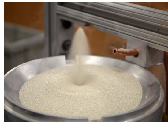
Zoom-in on diamond fountaining, with gas stream to sample particles
