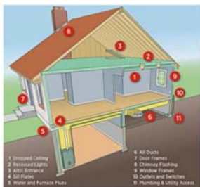
Sources of Air leaks in a Single-Family House (Source: DOE-Tips on Saving Money & Energy at Home 2011)
