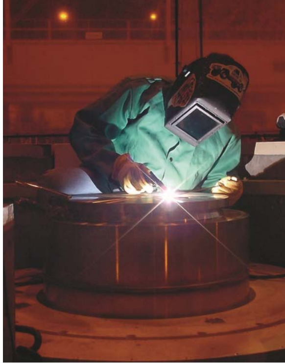
Figure 2. Arc welding of a DCSS canister provided by Fluor.
