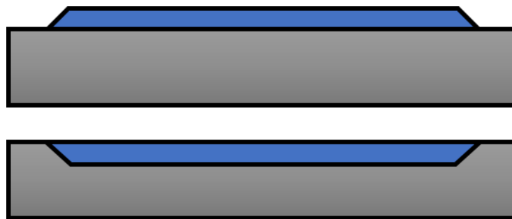
Figure 13. Coating strategies for localized coatings. Top: deposited coating without groove or blend. Bottom: grooved and blended coating.
