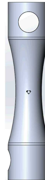
2 mm Through-hole Corner Cube Void
