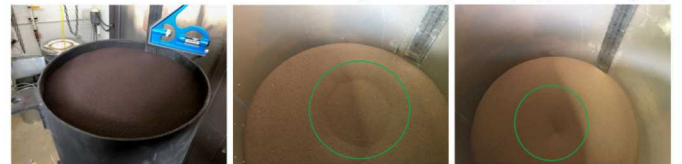
FIGURE 8: (left) initial height of high-fill test bin (mid) crater emerges and diameter shrinks with time (right) crater diameter converges to a point at the intersection of the flow channel and the wall.
