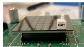
Fig. 2. (6mm) 3 organic glass cube coupled to a SiPM array pixel.
