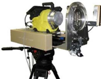
Figure 2. GeGI™ with ORNL coded aperture mask
