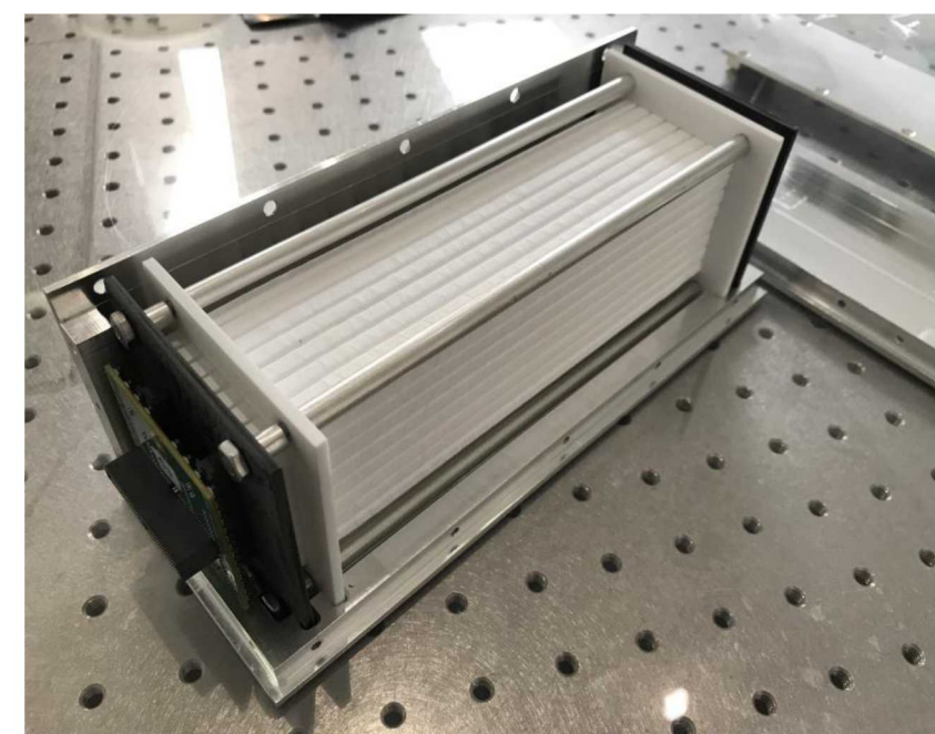
Optically-segmented single volume scatter camera prototype at University of Hawaii (photo credit: N. Kaneshige)
