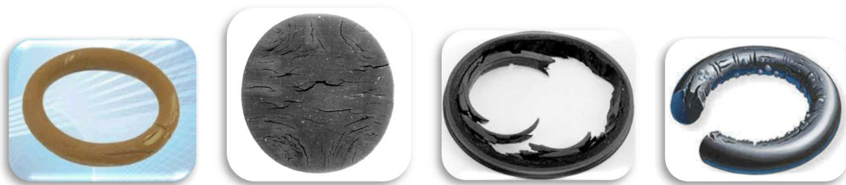
Figure 3. Examples of failures in elastomers in sCO 2 service due to explosive decompression
