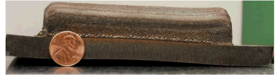
LENS 304L Build, T. Palmer (PSU) and D. Adams (SNL)
