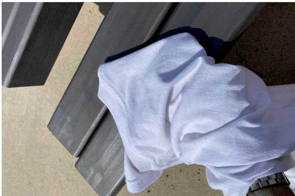
Figure 18. Rubbing a white T-shirt on the dark-coated surface of a DS-41 steel tube member
