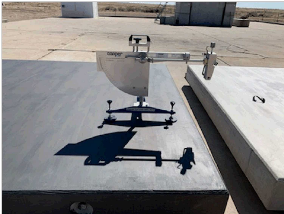
Figure 28. Typical concrete skid-resistance measurement setup
