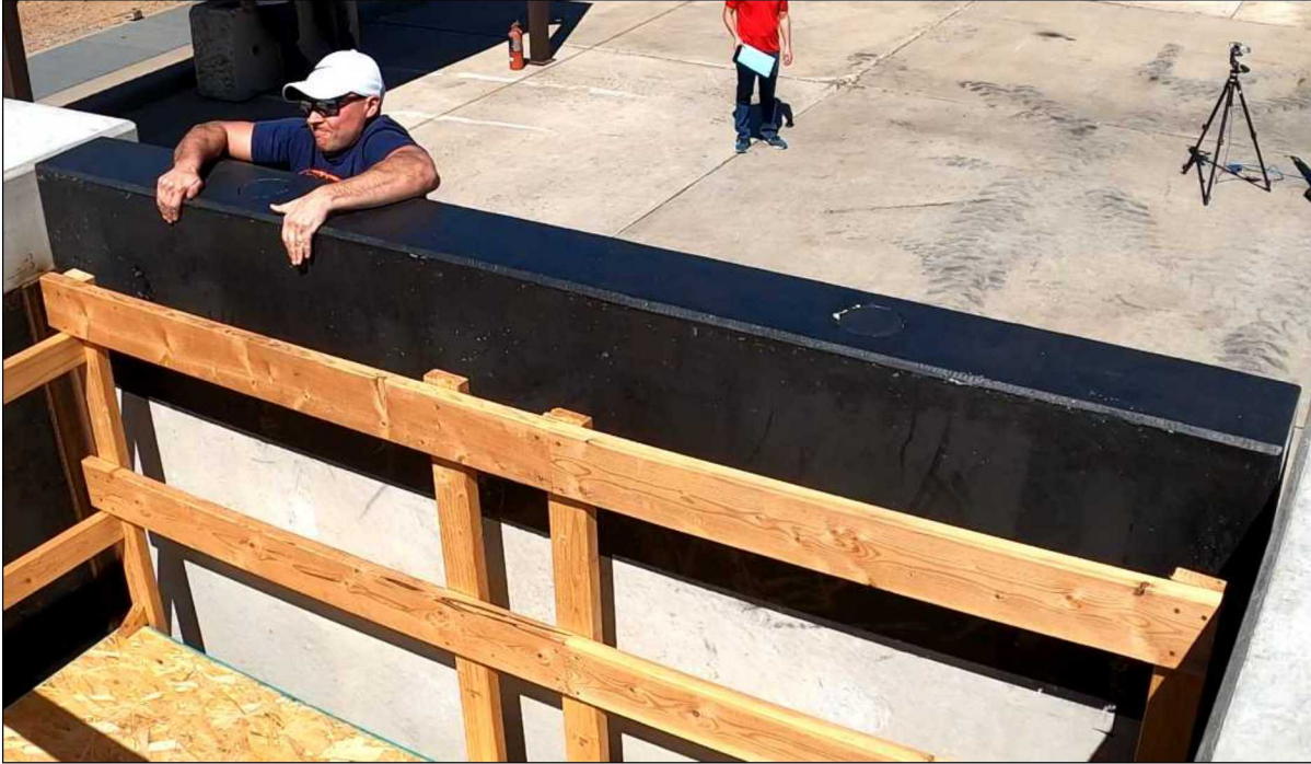
Figure 9. Scenario 1 role player attempting to defeat the dark base concrete wall
