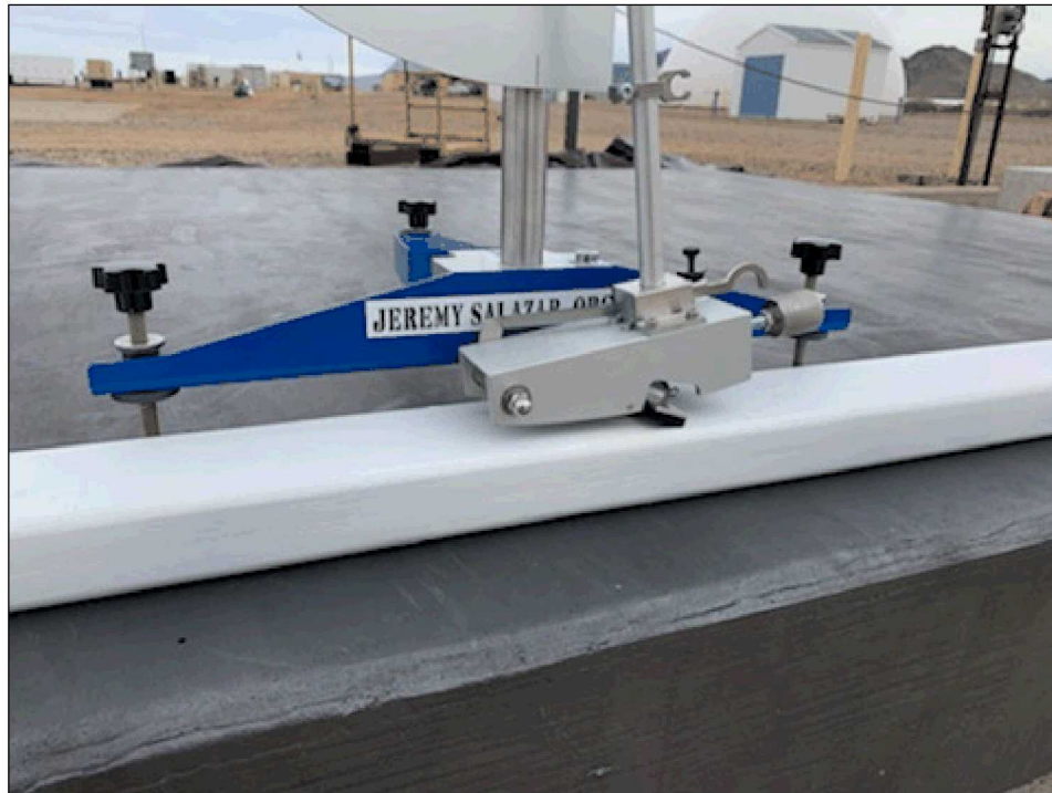
Figure 27. Typical steel beam skid-resistance measurement setup
