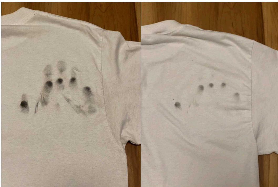
Figure 20. Pre- and post-wash views of the dark coating stain on a white T-shirt
