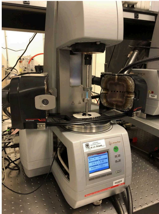
Figure 2-7. An Anton Paar Modular Compact TwinDrive rheometer taking measurements on a Model 2 elastic strap sample
