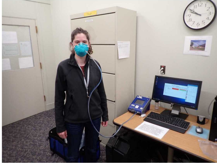
Figure 2-4. N95 respirator being tested by the PortaCount. The tester will provide a quantitative fit factor that scores the filtration efficacy, the respirator seal, and the ability of our industrial hygiene team to don the machine.
