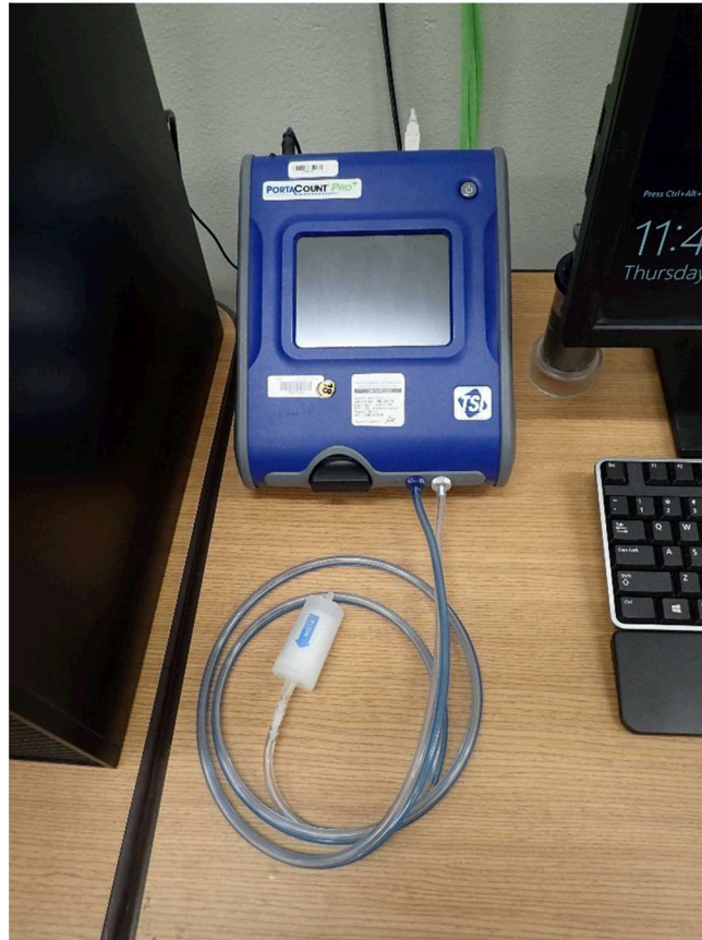
Figure 2-3. TSI PortaCount Pro+ Respirator Fit Tester Model 8038
