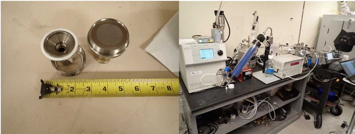
Figure 2-11. The stainless steel housing for a circular punch of respirator filter (left). The FPT system (right)
