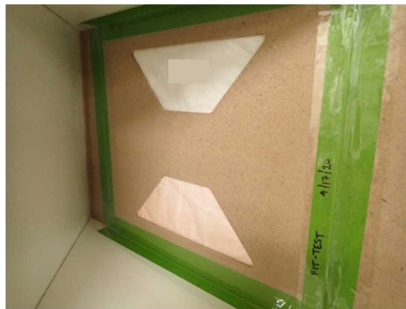
Figure 2-10. The pouch/duck-bill style respirator split and mounted into a filtration box for the large-scale filtration testbed
