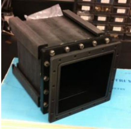
Fig. 27. 3D printed plastic waterproof enclosure
