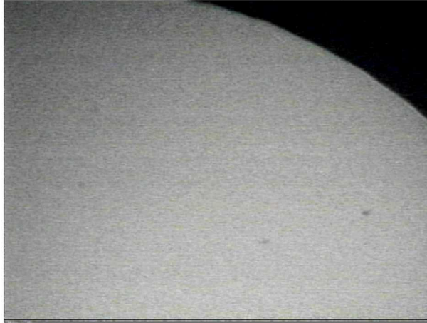
Evaporated Titanium Film on Quartz Witness (metallic appearance)
