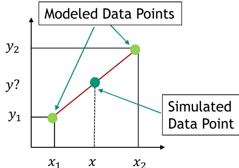
1. Find two modeled data points that bracket the simulated data point.
