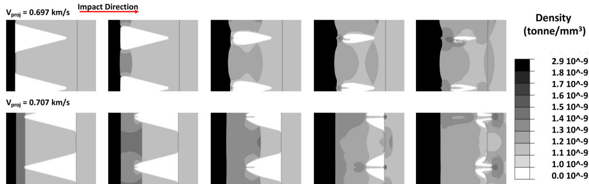
FIG. 7. Density contours predicted for the shock propagation in a wedge geometry with an impact direction from left-to-right (top) and right-to-left (bottom) at 0.697 km/s and 0.707 km/s, respectively.
