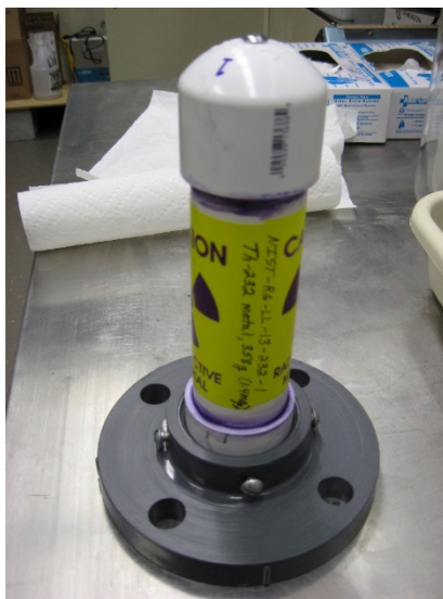
Figure 16-4. NIST traceable thorium bar source.
