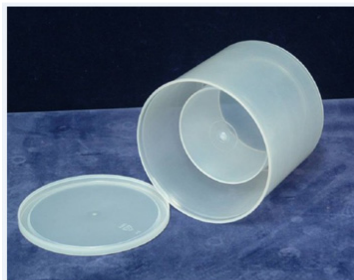
Figure 5-3. Photo of Marinelli container. [9]
