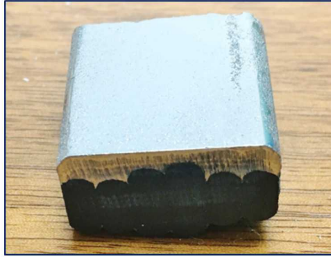
Figure 16: Sample of metallized BAAM Polymer with a Zinc bond coat that has been machined flat, followed by a polishing “Amorphous Alloy” top coat.
