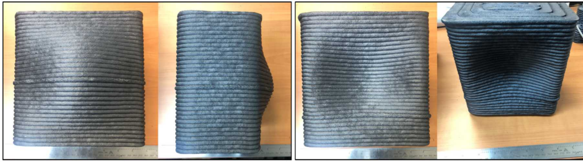
Figure 22: Convex (Left) and Concave (Right) simple geometry tooling blocks BAAM printed in PPS/CF-50%.
