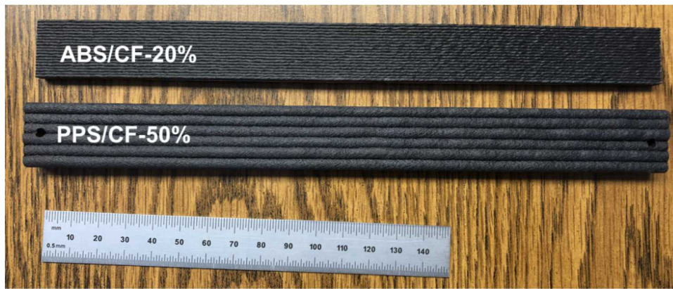
Figure 4: Image of ABS/CF-20% and PPS/CF-50% BAAM substrates to be used for spray trials.
