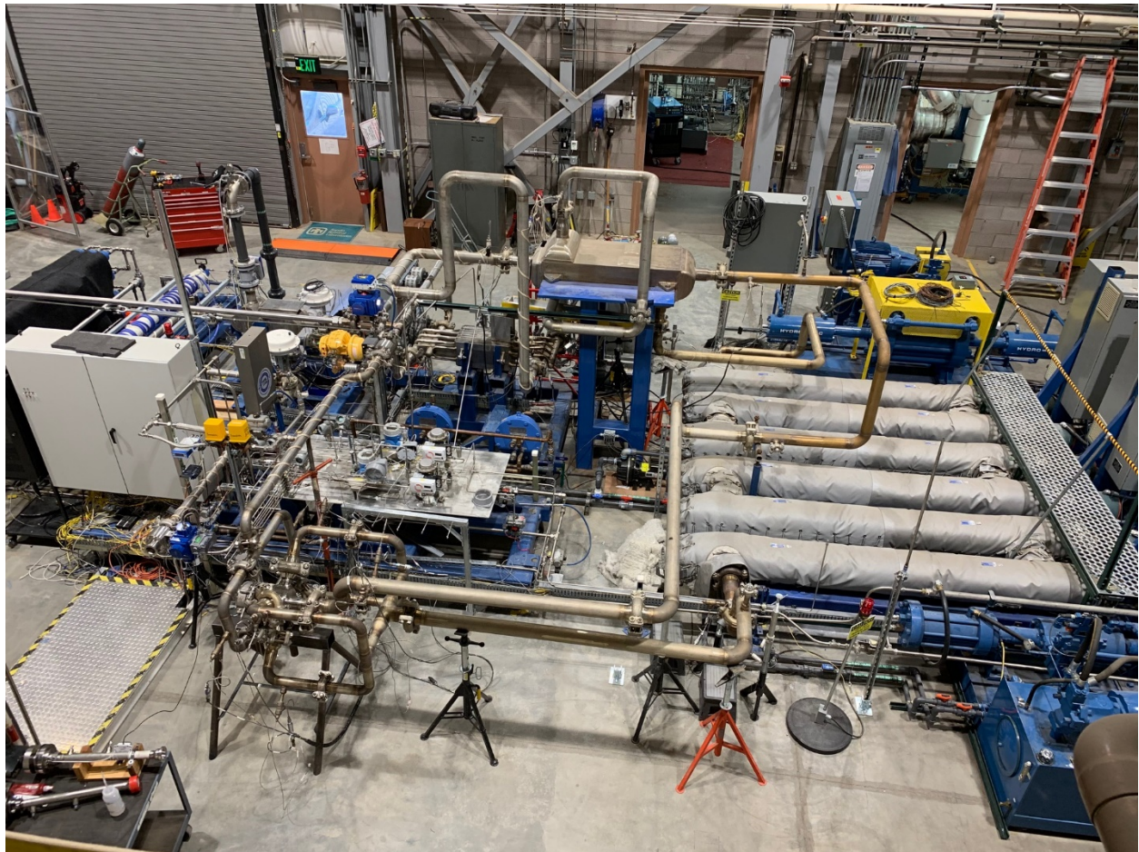
Figure 1. Development Platform with insulated heaters on right, turbomachinery in foreground, and heat exchanger train in background
