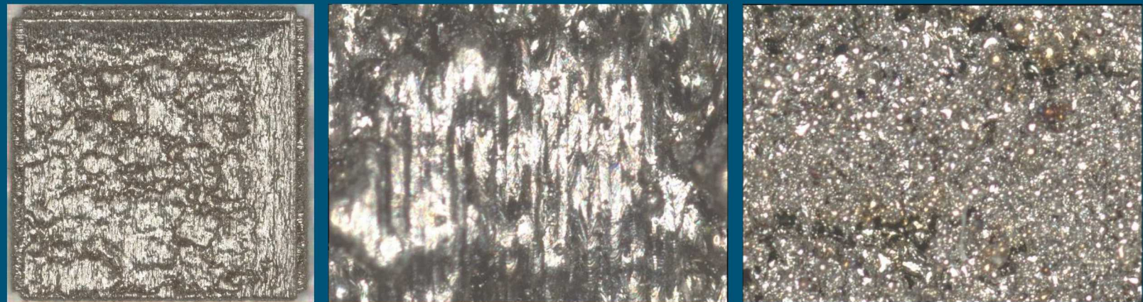
60.1W, 300mm/sec 891 \mu m Pkk form (left), top 73.8 \mu m Sa roughness (center), side 38.1 \mu m Sa roughness (right)
