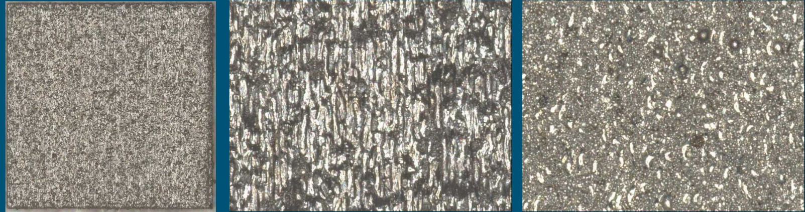
100.2W, 1500mm/sec 209 \mu m Pkk form (left), top 13.5 \mu m Sa roughness (center), side 9.98 \mu m Sa roughness (right)
