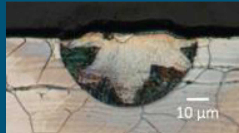
melt pool on plate, 100W, 1500 mm/s
