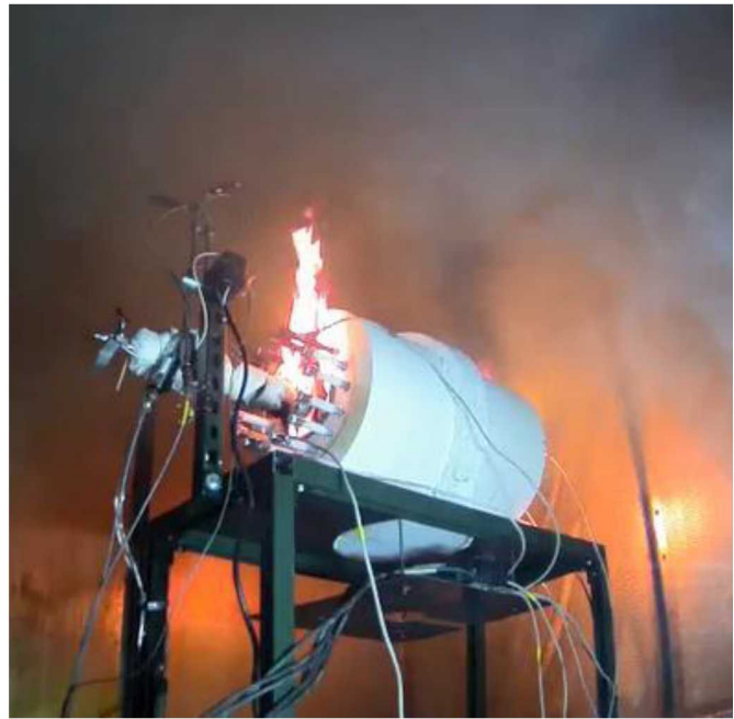
Figure 23. Configuration 5 Post-test PCV and Video Image Showing Flames During Test.
