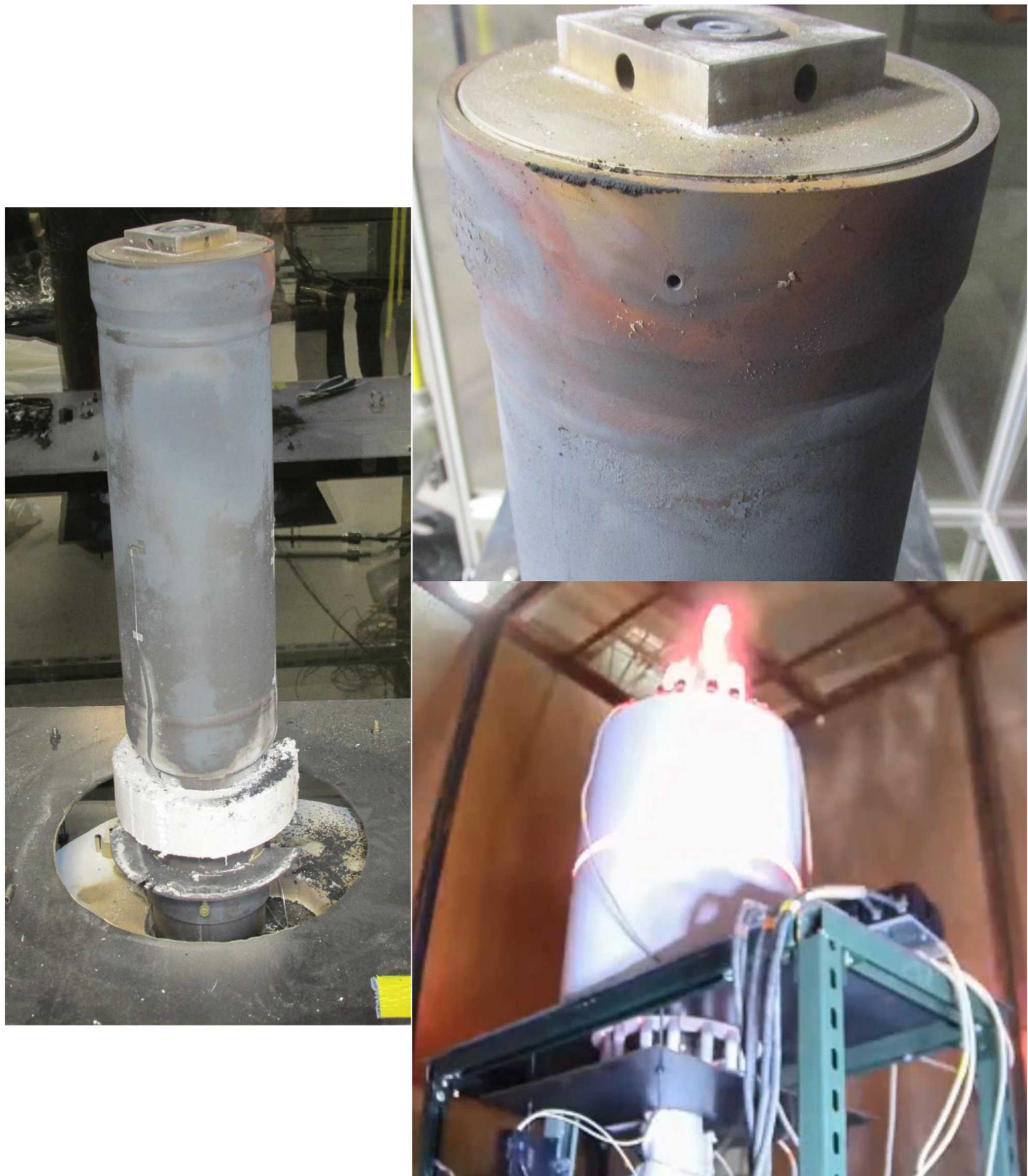
Figure 13. Configuration 1 Post-test PCV and Video Image Showing Flames During Test.
