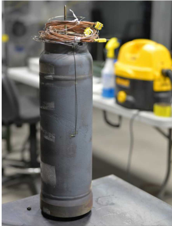
Figure 23. Configuration 5 Post-test PCV and Video Image Showing Flames During Test.
