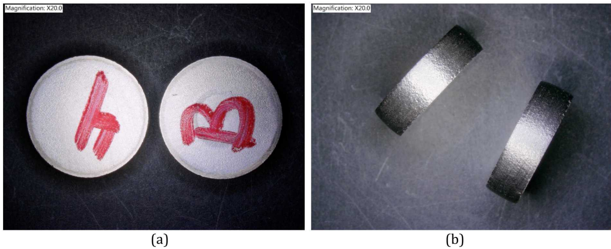
Figure 73. Pictures of the wrought specimens after dynamic compression tests. (a) end surfaces; (b) side surfaces.
