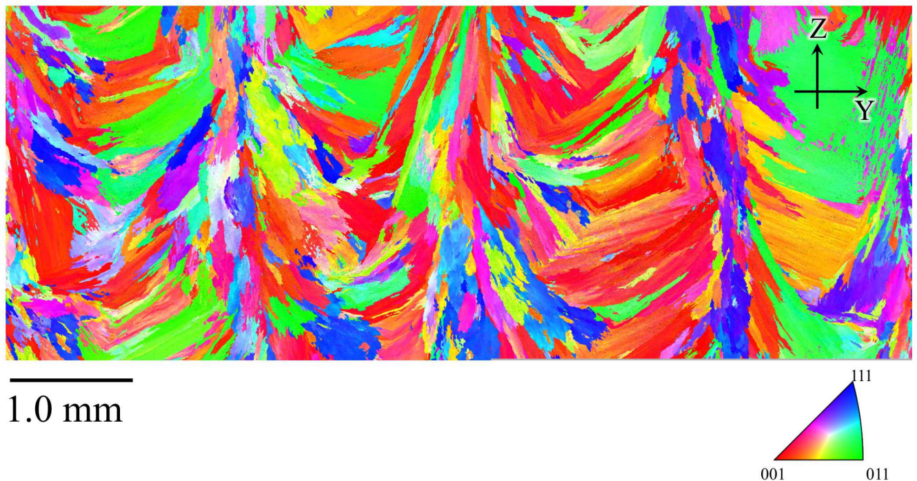
Figure 17. Large area view of microstructure of AM SS 304L made using a laser power of 3.8 kW implementing parallel scan method for fabrication. Crystal orientation maps show evidence of multiple layers used in building. The colors coordinate the (hkl) orientations of grains with their x (i.e., left-right) direction as shown.
