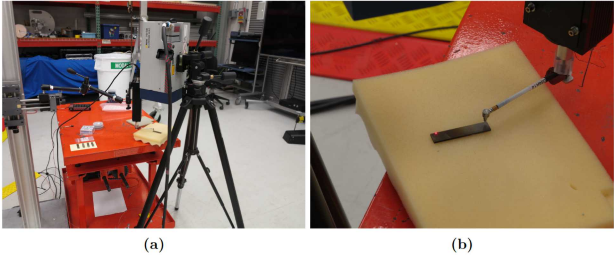
Figure 60. Test setup showing (a) the laser vibrometer and (b) impact hammer setup.
