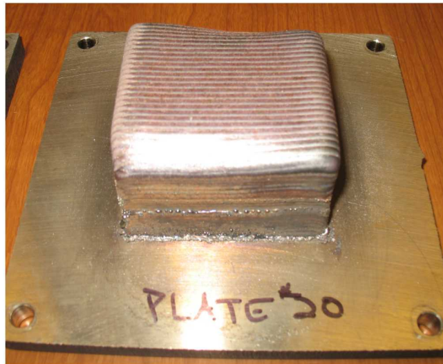
Figure 9. Photograph of square bar made for producing high impact gas gun test samples. The second sample is shown in Appendix 13.2.
