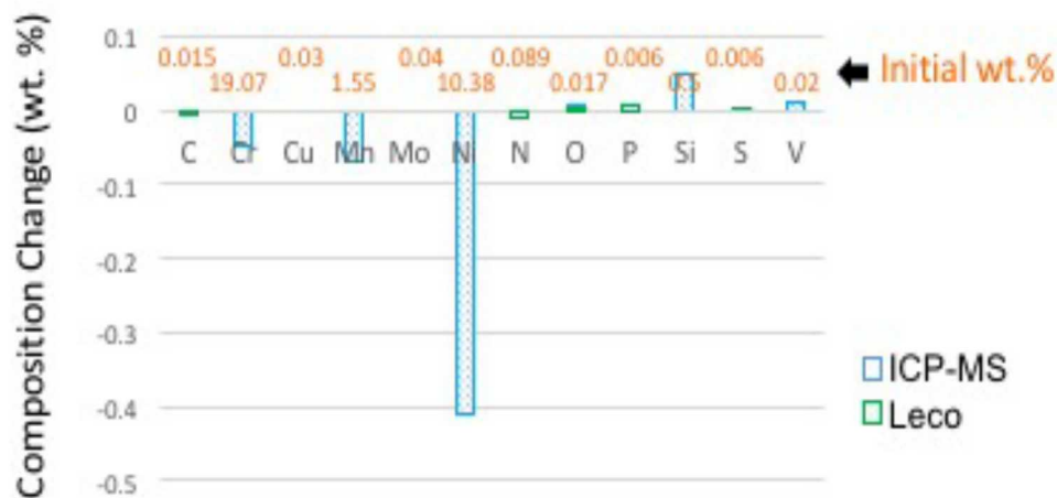
Figure 13 Compositional changes of deposited material referenced to powder used. These are results from AM using a P_{avg} = 2.0 kW.
