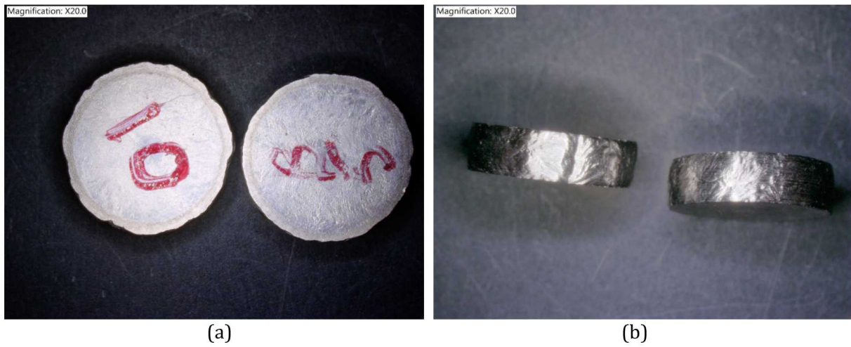
Figure 76. Pictures of the 2.0 kW, cross-hatched AM steel samples (not heated after deposition) after compression tests. (a) end surfaces; (b) side surfaces.
