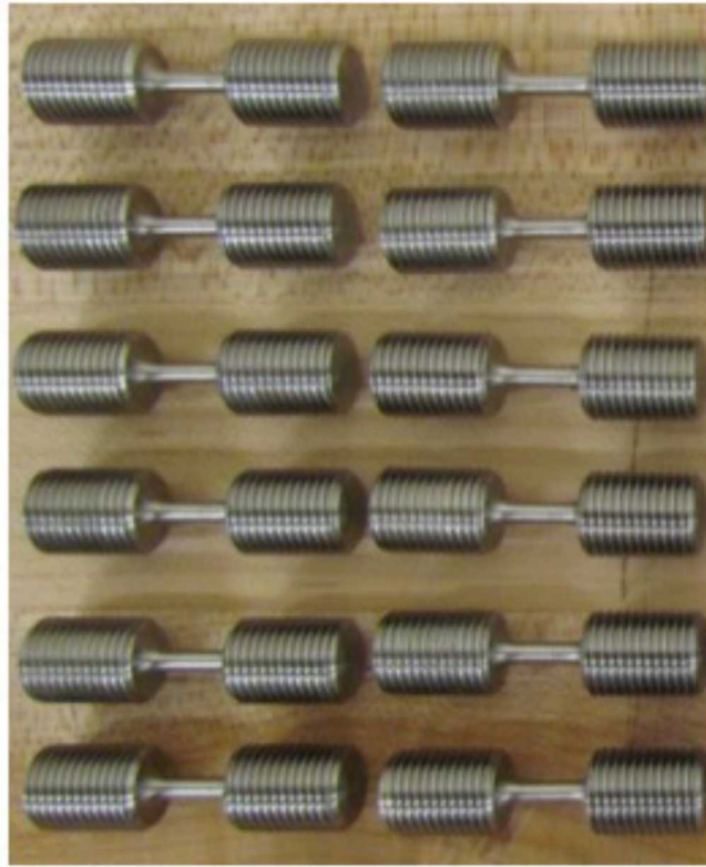
Figure 33. Photograph of machined tensile samples for Hopkinson tests. Samples are 4.572 cm. (1.80 in.) long.
