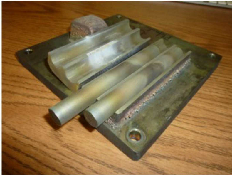
Figure 32. Photograph of cylinders extracted by electro-discharge machining.
