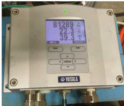
Figure 5 Vaisala Temperature Monitor within FACT Bunker
