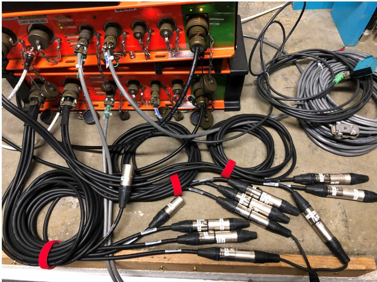
Figure 25 Input Shorted Offset Configuration Picture
