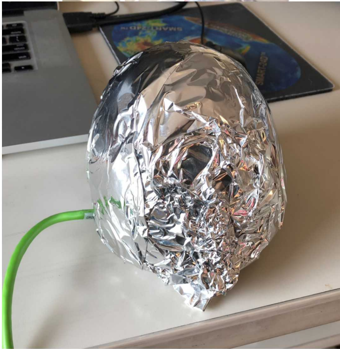
Figure 113 GPS and PTP antennas covered for drift test
