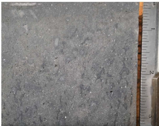
Figure 11. Cement sample sliced parallel to the long axis, reflected light.
