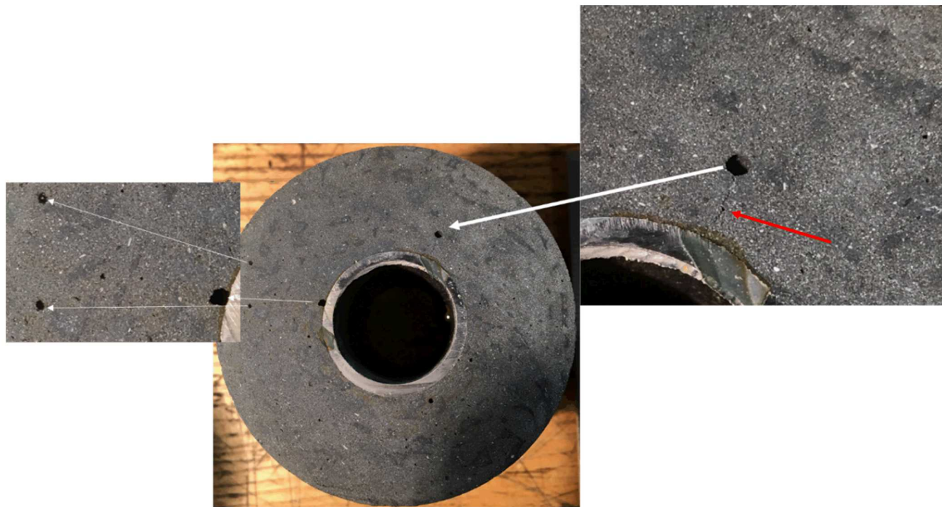
Figure 12. Cement sheathed steel sample sliced perpendicular to the long axis, reflected light.
