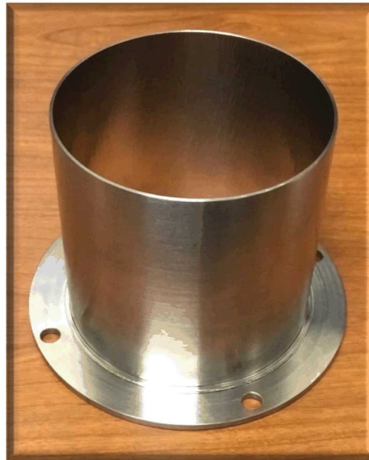
Hybrid Additive Subtractive Ti6Al4V
