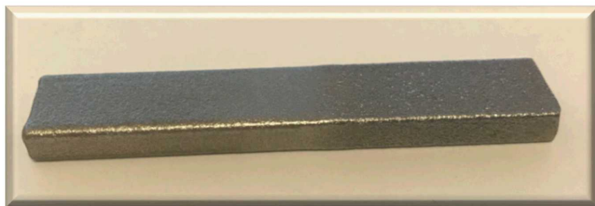
Multi-material ½ magnetic steel ½ non-magnetic steel
