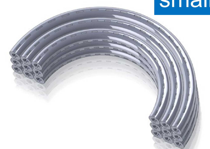
Radius of curvature 636.62 microns Length of waveguide 2 mm Waveguide diameter 5 microns
