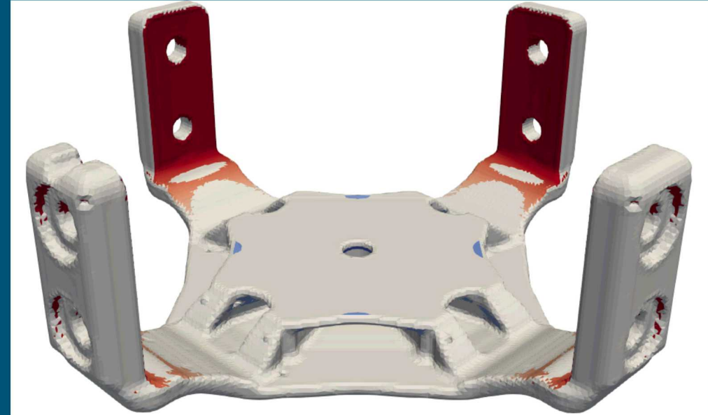
Design courtesy of Clinton Holtey using Plato. Displacement predictions by Kyle Johnson. Red = 0.1 mm.
