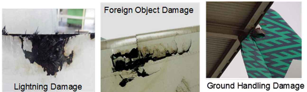
Figure 2-2: Sample Sources of Damage to Composite Structures
