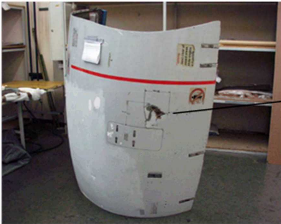
Figure 2-3: Sample Damage From Ground Service Vehicle Impact
