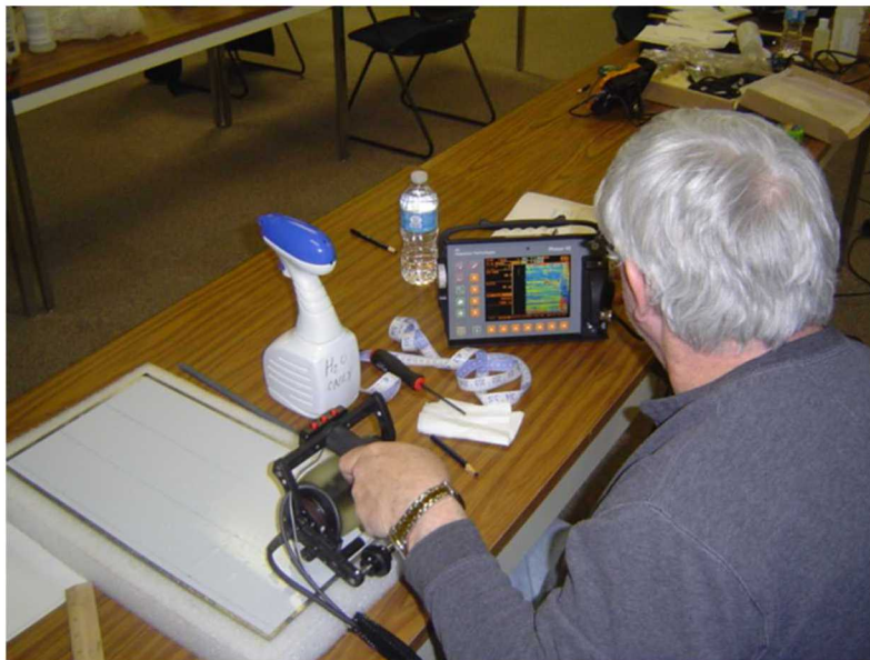
Figure 3-21: Deployment of RotoArray Wheel Probe on a Composite Laminate Test Specimen in the AANC Flaw Detection Experiment
