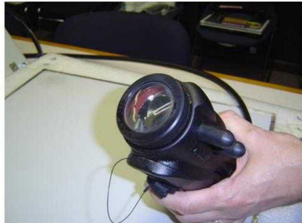
Figure 6-54: Deployment of AcoustoCam Video-Based UT System on Solid Laminate POD Experiment
