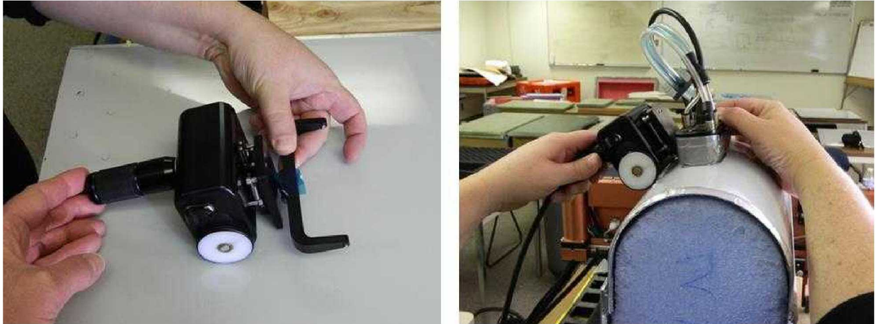
Figure 6-36: Use of Different Linear Array Probes and Encoders to Inspect Various Test Specimen Geometries
