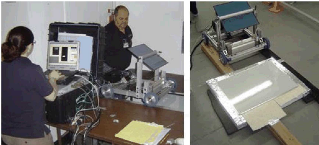
Figure 6-83: Deployment of Mistras Line Scanning Thermography System on Solid Laminate POD Experiment
