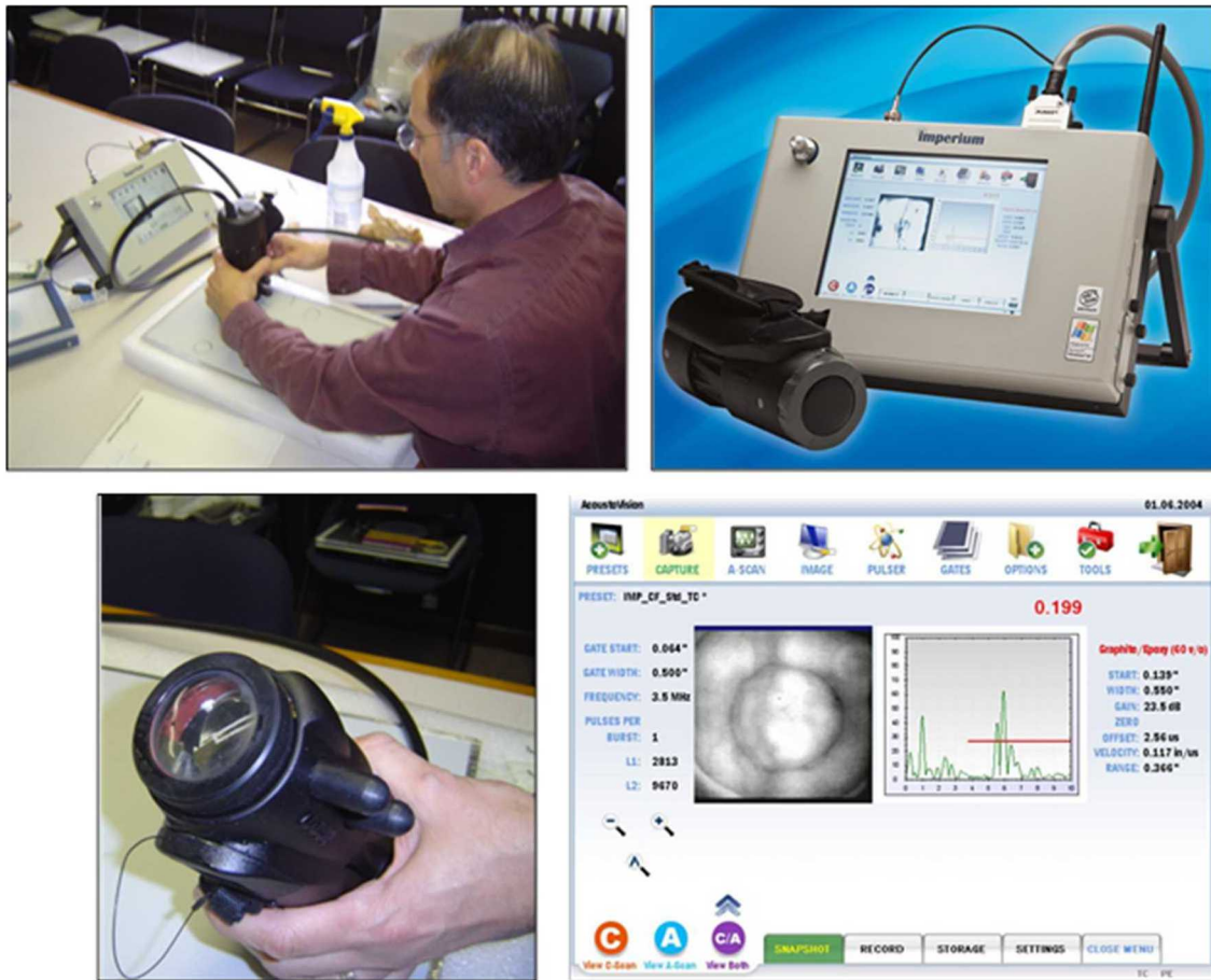
Figure 3-41: Imperium Acoustography Equipment and Flaw Image
