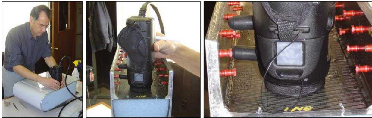
Figure 6-55: Photos Showing Some Restriction in AcoustoCam Movement Within the Confined Spaces Present on Bullnose Specimens (Spar Cap Channel Region)
