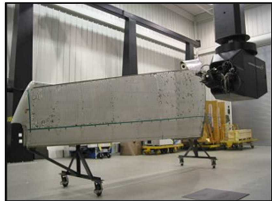
Figure 3-30: Schematic of Laser UT Method and Deployment in Gantry System and Rail System
