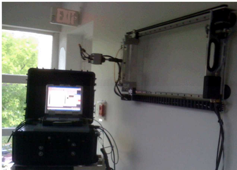
Figure 3-74: Mistras Line Scan Thermography System – Small Area Scanner
