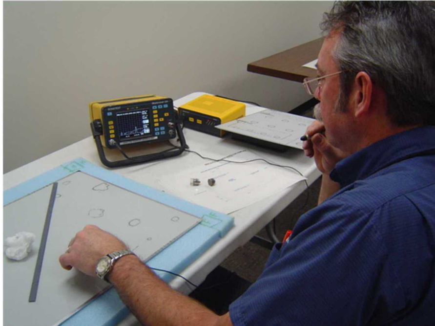
Figure 5-4: Inspector Completing Inspection and Marking Flaw Detection on the Test Specimen
