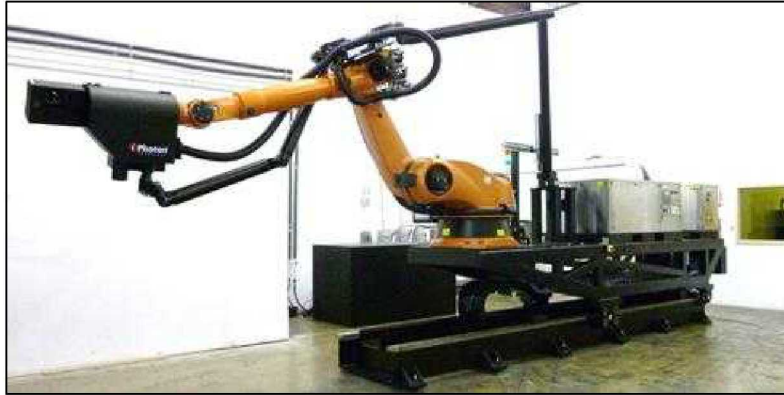
Figure 6-47: iPhoton Laser Ultrasonic Gantry-Based Inspection System
