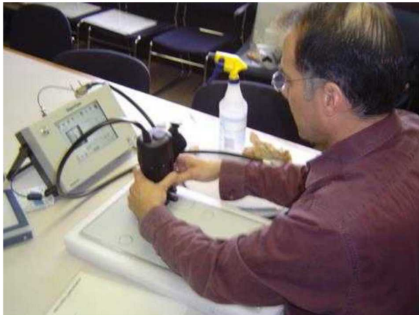
Figure 6-54: Deployment of AcoustoCam Video-Based UT System on Solid Laminate POD Experiment
