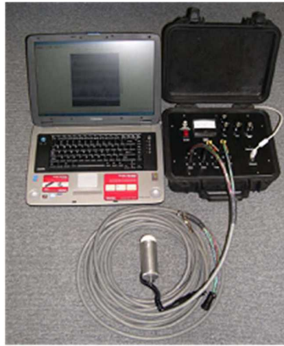
Figure 3-48: Basic Equipment Set-up for Microwave Inspection
