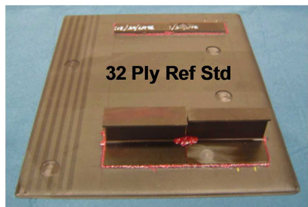
Figure 4-7: 20 and 32-Ply NDI Feedback Specimens (backside view) Used by Inspectors Prior to Starting the Blind POD Inspections
