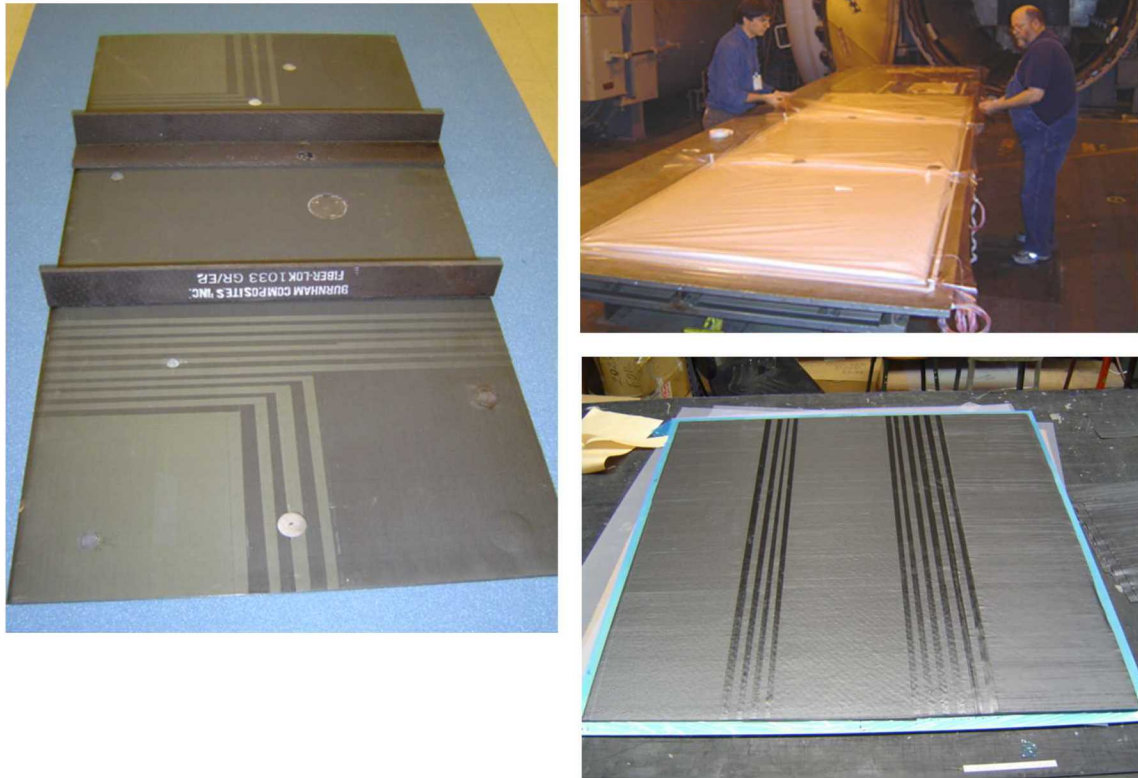
Figure 4-20: Layup of Composite Laminates with Simple Taper and Complex Taper and Bonding of Substructure Elements
