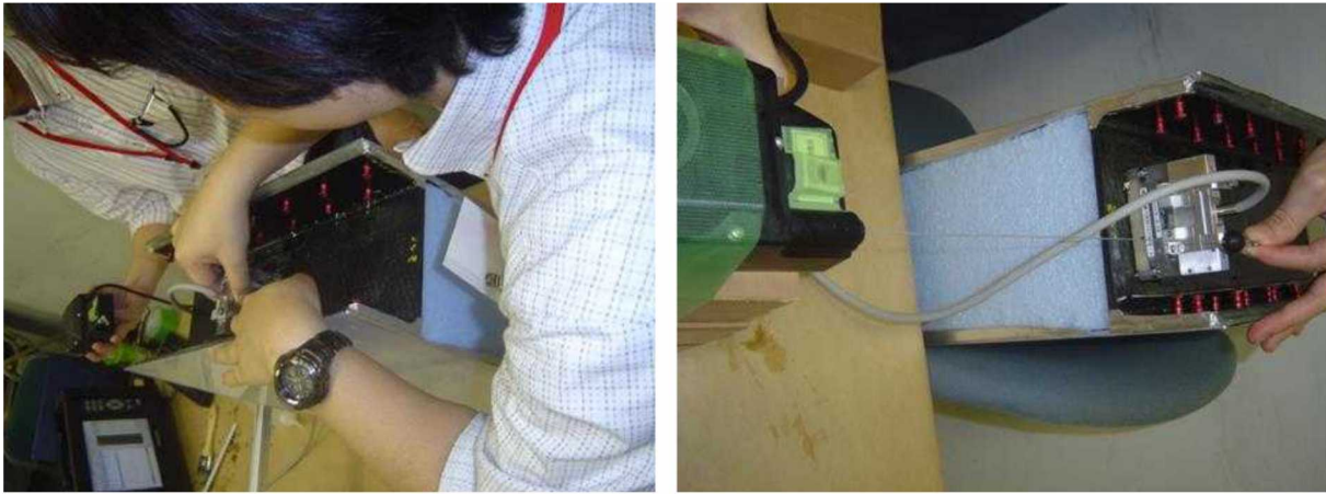
Figure 6-29: Use of Different PA-UT Array Probes and Encoders to Inspect Various Test Specimen Geometries
