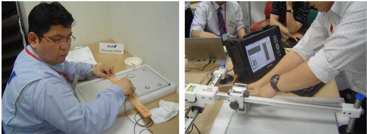
Figure 6-93: Deployment of MatrixEye Phased Array UT System by All Nippon Airways on Solid Laminate POD Experiment
