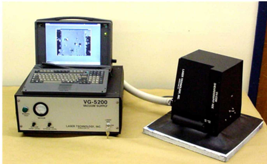
Figure 3-51: LTI-5200 Portable Shearography System with Camera on Test Specimen
