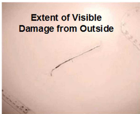
Figure 2-10: Example of External Impact Creating Minor Surface Demarcation But Significant Internal Damage
