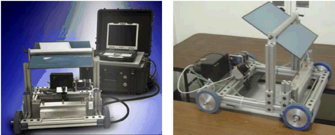
Figure 6-82: Mistras Line Scanning Thermography THELIS-P Device
