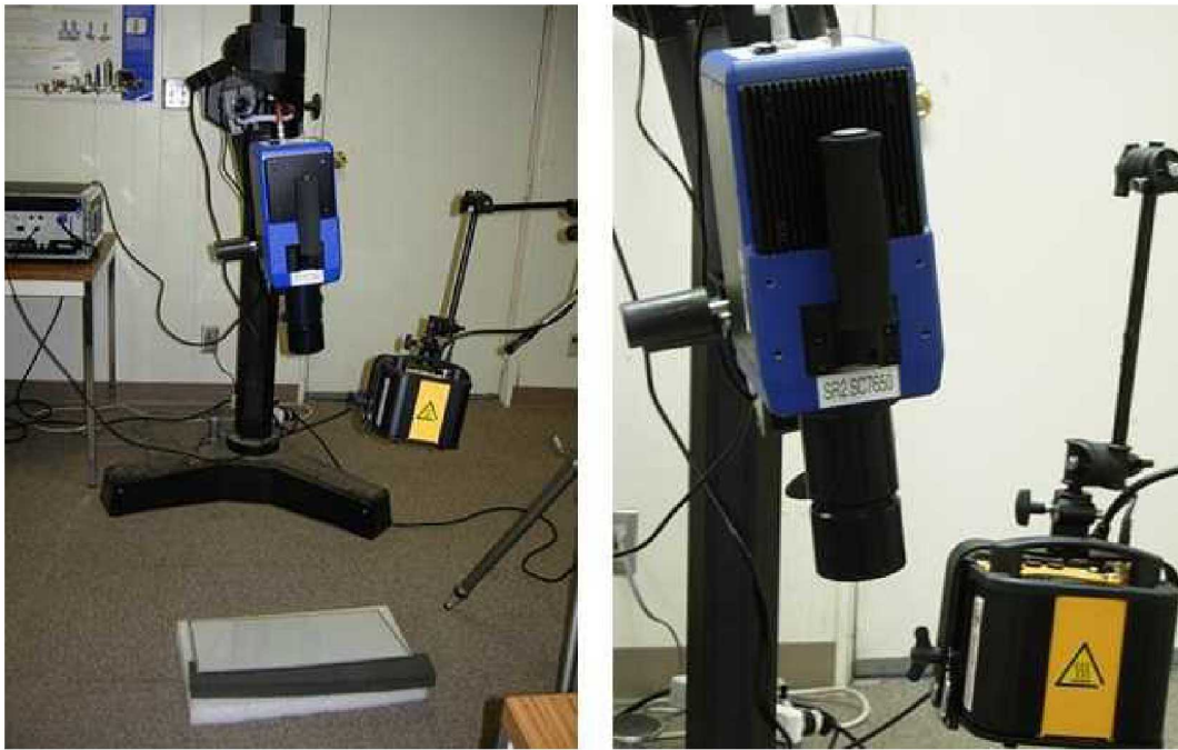
Figure 6-87: MovieTherm Lock-In Thermography Device
