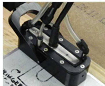
Figure 3-16: FlawInspecta Linear Array UT System Deployed on MAUS V Scanner Platform – Linear Array UT Probe Includes a Delay Line Shoe
