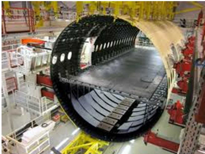
Figure 1-6: Production of an All-Composite Fuselage Section
