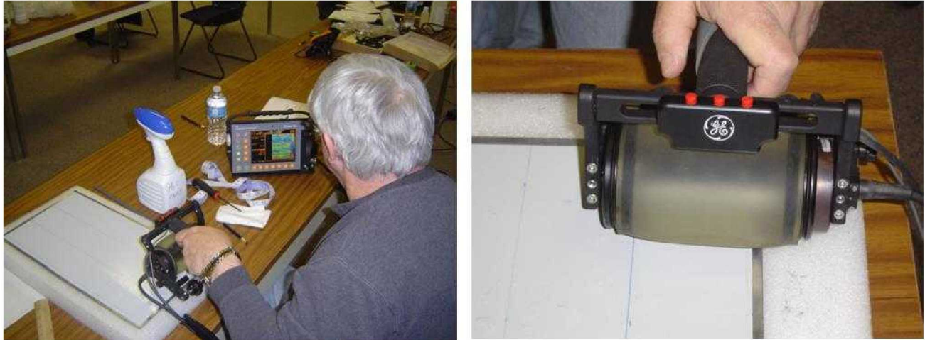
Figure 6-40: Deployment of General Electric Phasor XS with RotoArray PA-UT System on Solid Laminate POD Experiment
