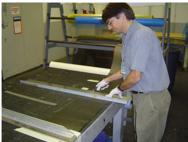
Figure 4-19: Solid Composite Laminate Flaw Detection Experiment – Test Specimen Fabrication
