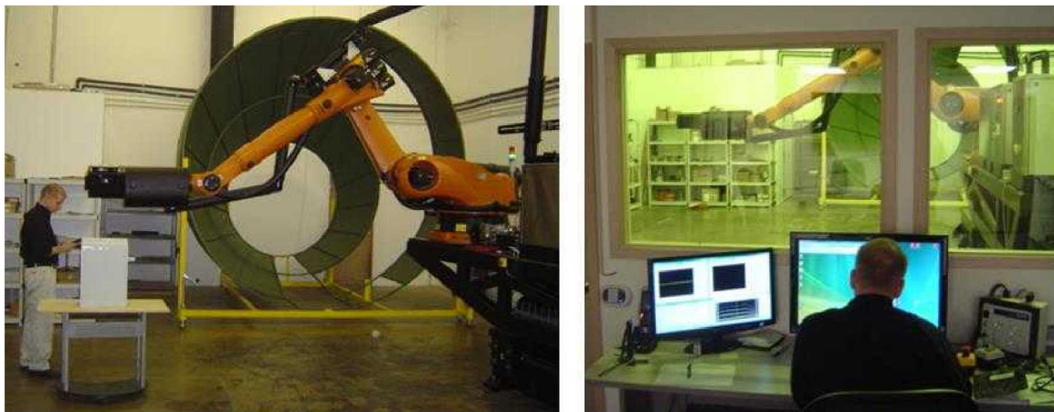
Figure 6-48: Deployment of iPhoton Laser Ultrasonic System on Solid Laminate POD Experiment
