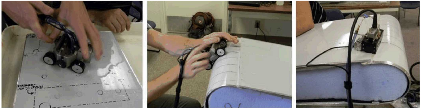
Figure 6-22: Use of Different PA-UT Array Probes and Encoders to Inspect Various Test Specimen Geometries
