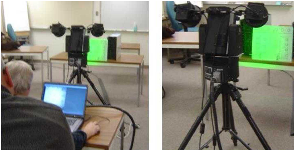
Figure 6-69: Deployment of LTI Shearography System (5100 HD) on Solid Laminate POD Experiment
