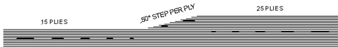
Figure 4-17: Trial Signal-to-Noise Solid Laminate Specimen for Preliminary Testing of Methods for Producing Engineered Flaws
