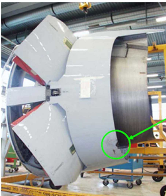
Figure 2-6: Sample Damage from Lightning Strike
