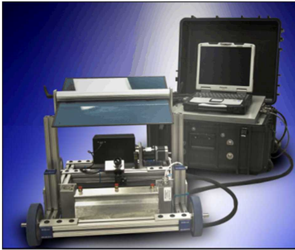
Figure 3-73: Mistras Line Scan Thermography System – Crawler Used on Composites
