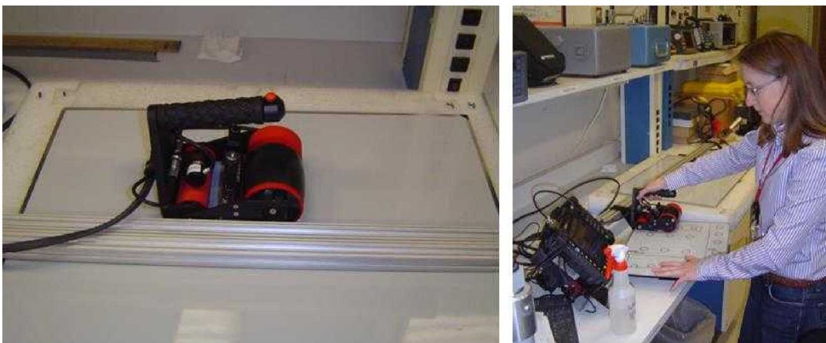
Figure 6-44: Deployment of Sonatest UT Linear ArrayProbe with OmniScan Unit on the Solid Laminate POD Experiment
