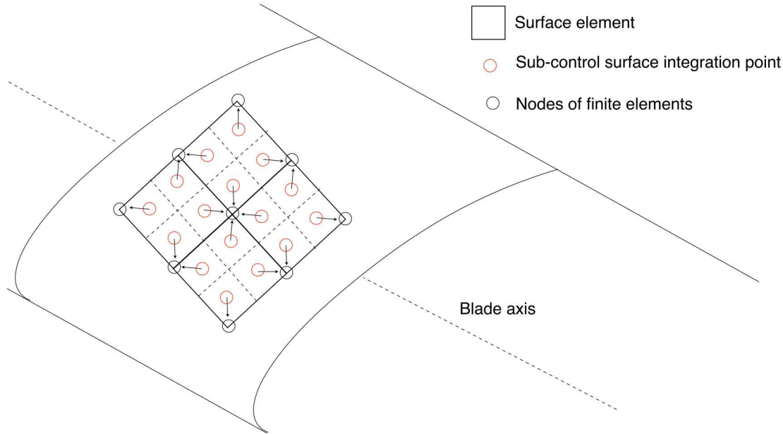
Figure 28: Assembly of loads on each surface element into point-loads on the nodes.
