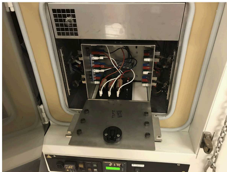
Figure 3. K2 Power cells sharing in a 30°C test chamber
