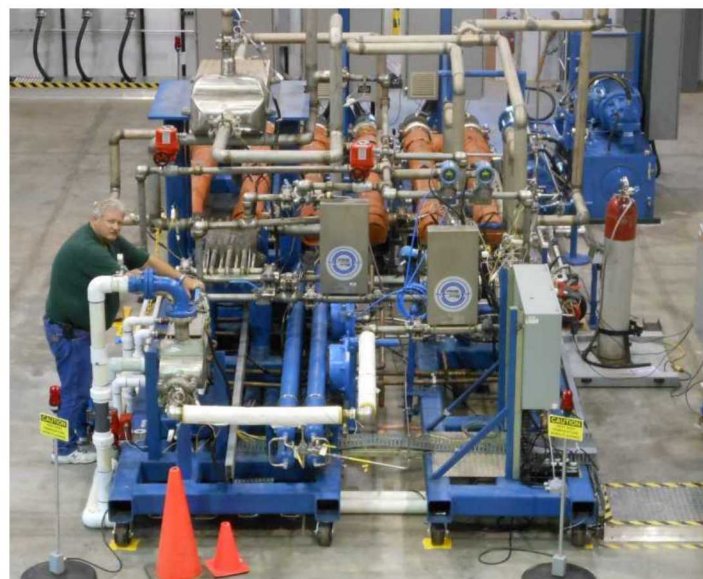
Figure 2. Recompression Closed Brayton Cycle: photos of the SNL Brayton Laboratory test assembly, with major components labeled
