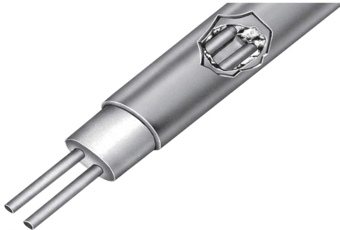
Figure 5: Mineral Insulated. Single or double (shown) resistance wires. MgO mineral insulation. Alloy metal sheath.
