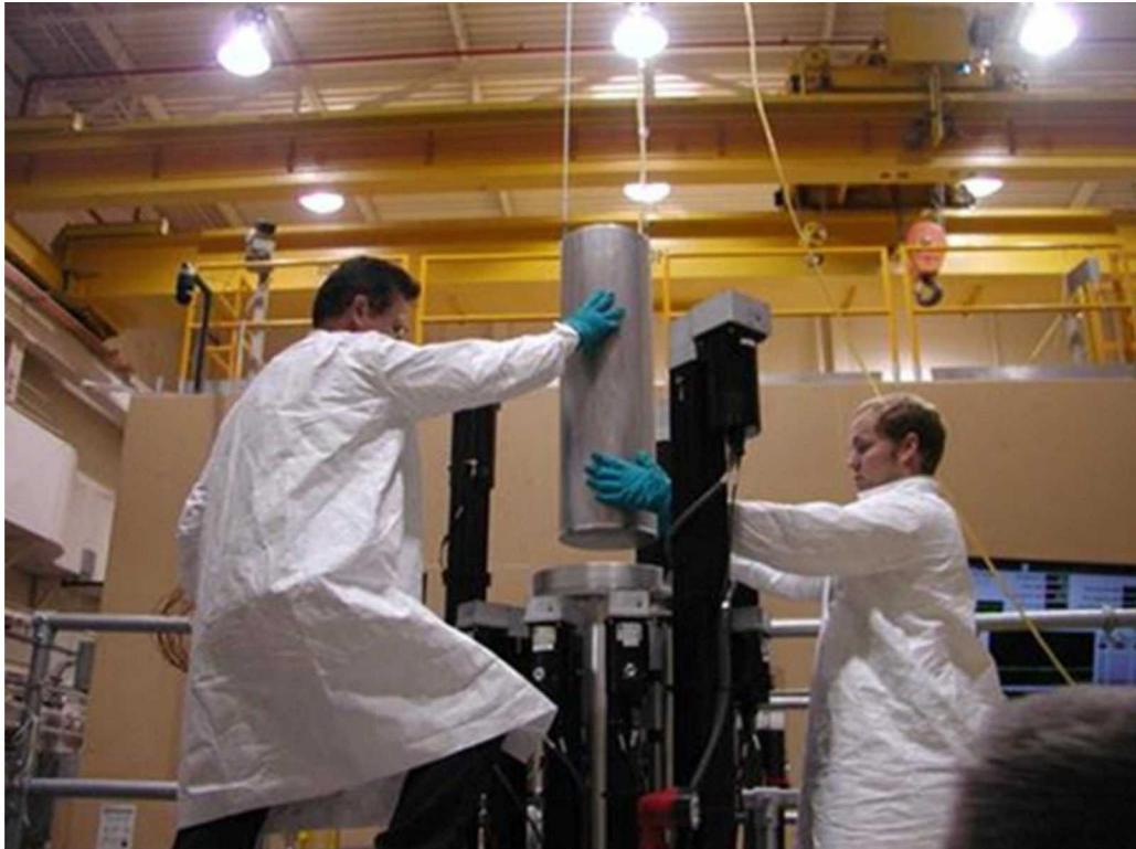
Figure 4. Experiment Package Loaded into the ACRR Central Cavity.
