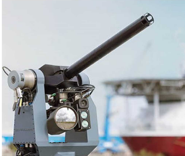
Figure 4-15: Example of a Kinetic Mitigation (net projectile) for Fixed-Site Application (Skywall 300)
