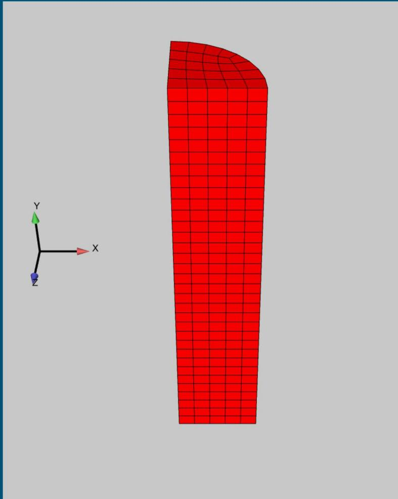
$\frac{1}{4}$  symmetry model with no normal displacement boundary conditions specified on symmetry planes
