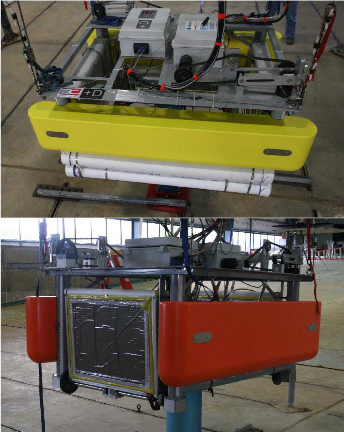
Figure 6-1. Phase 1, Additional buoyancy provided by PVC pipes (top); Phase 2, Additional buoyancy provided by new floats (bottom)
