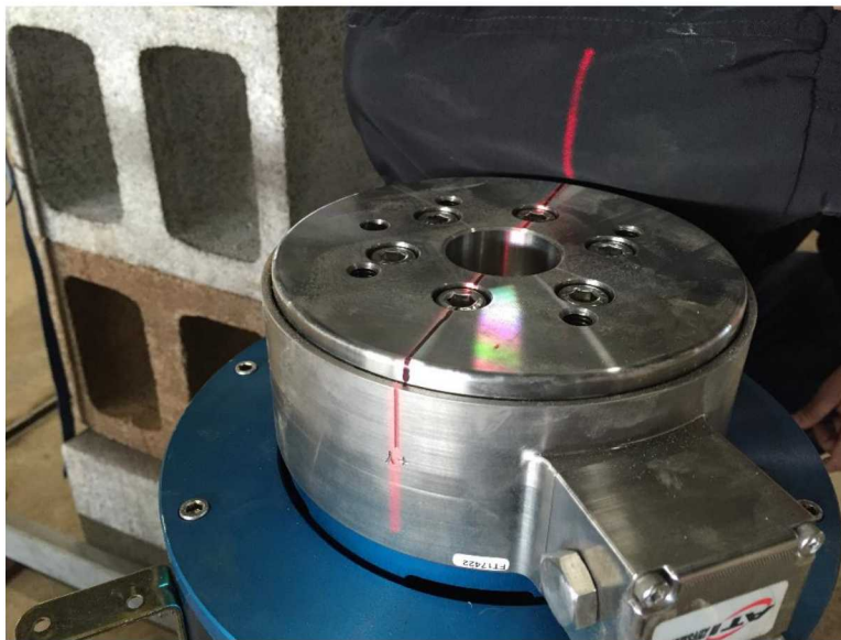
Figure 5-6. 6-DOF Load Cell between Arm and FOSWEC
