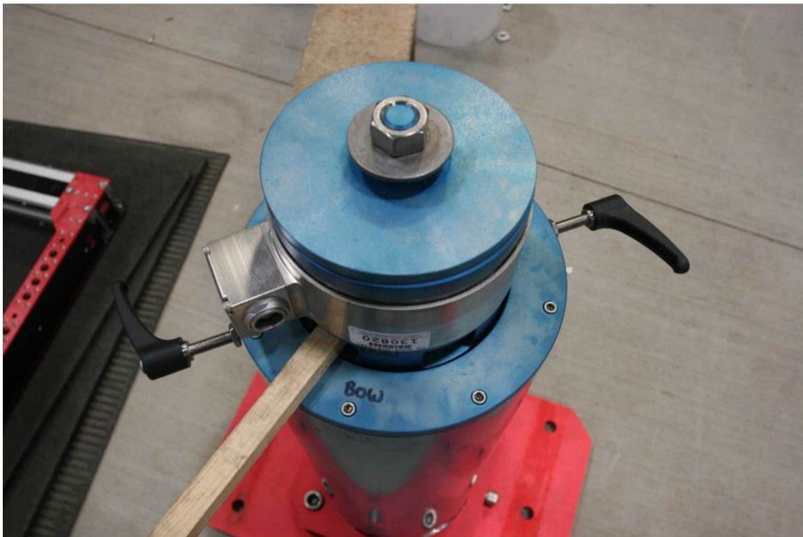
Figure 6-4. Heave Constraint Modification
