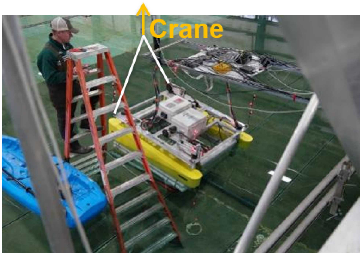
Figure 5-11. Pitch Decay and Static Offset Setup
