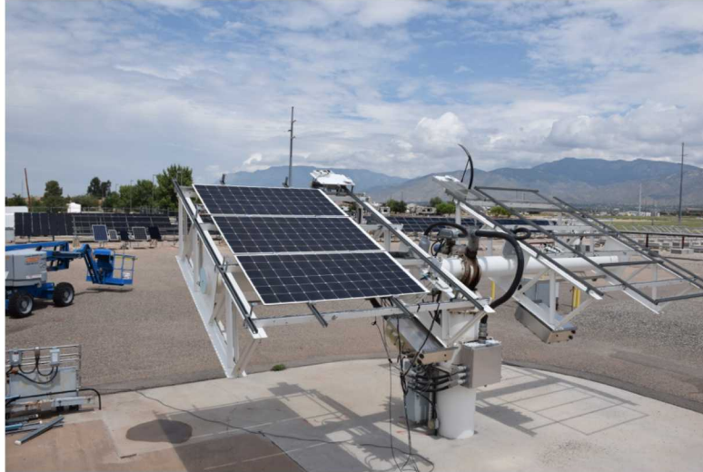
Figure 5-3. Test Devices mounted on two-axis solar tracker
