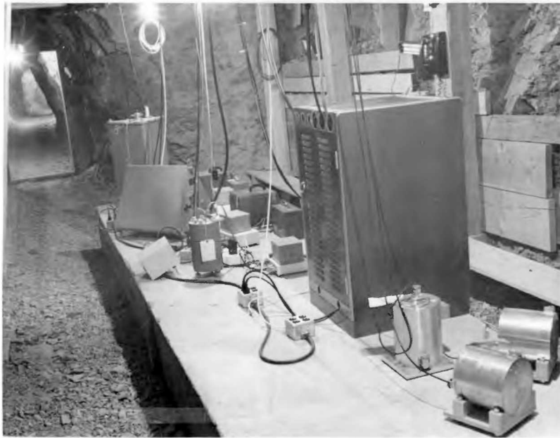
Figure 2. Early 1970s photo of the installation at Nelson, NV. All the LSBN stations were installed on poured-concrete seismic piers in abandoned mines.
