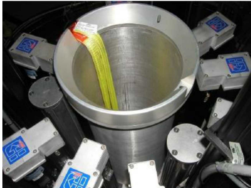
Figure 2. The top loading area of the 9-inch dry central cavity.
