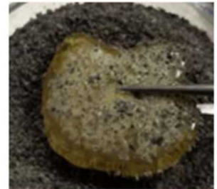
(b) PbO reacted in 22 °C dolomite of sizes between 0.3 and 1 mm (3D test)
