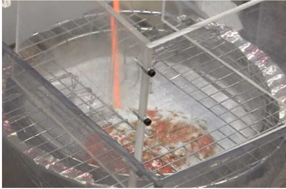
Figure 4. 1 kg PbO at 950 °C pouring onto < 1mm calcite bed on a pan (090418 test).
