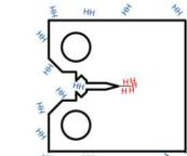
**Fracture resistance of pipeline steels in H2 is greater than driving force on semi-elliptical cracks**
